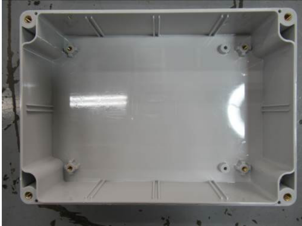
There is no trace of water inside.
