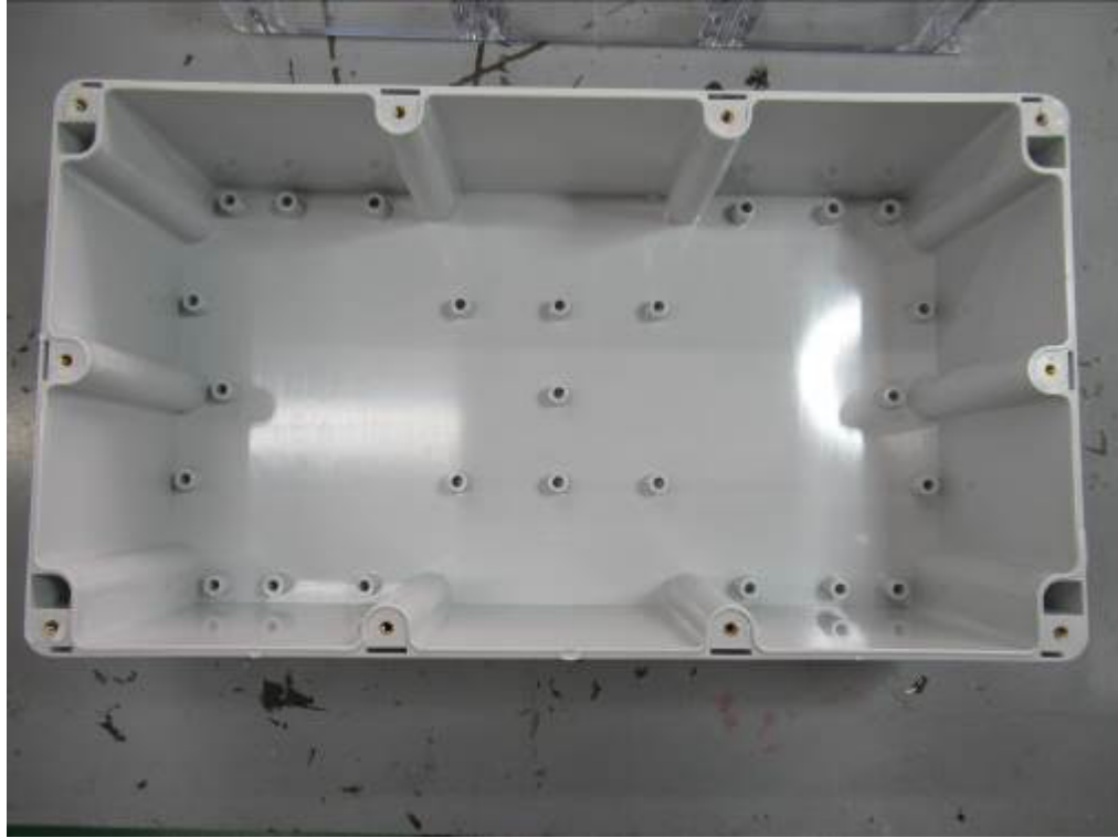
There is no trace of water inside.
