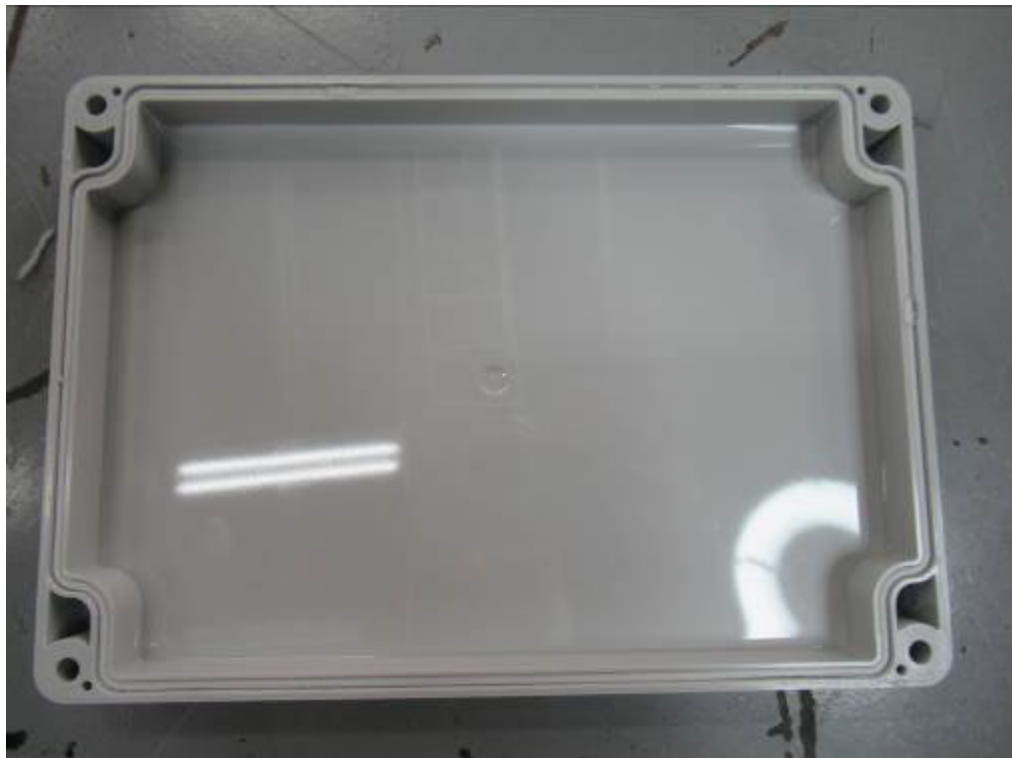
There is no trace of water inside.
