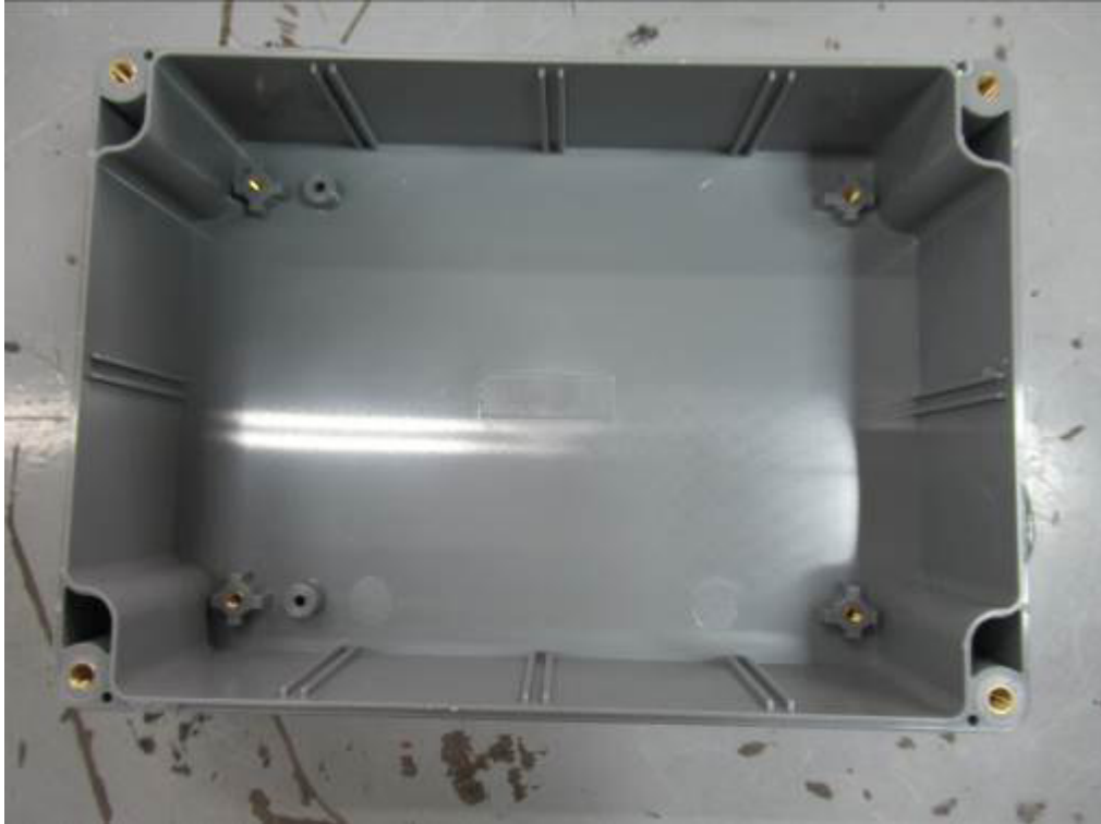
There is no trace of water inside.
