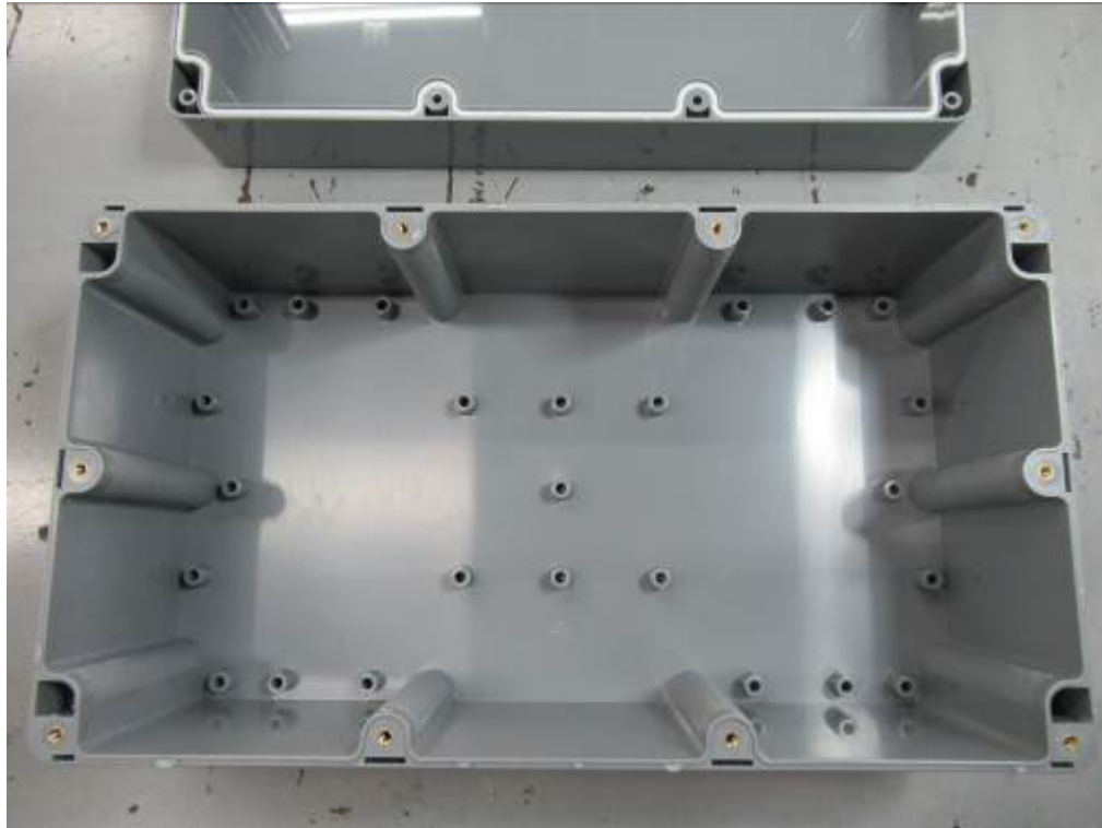
There is no trace of water inside.
