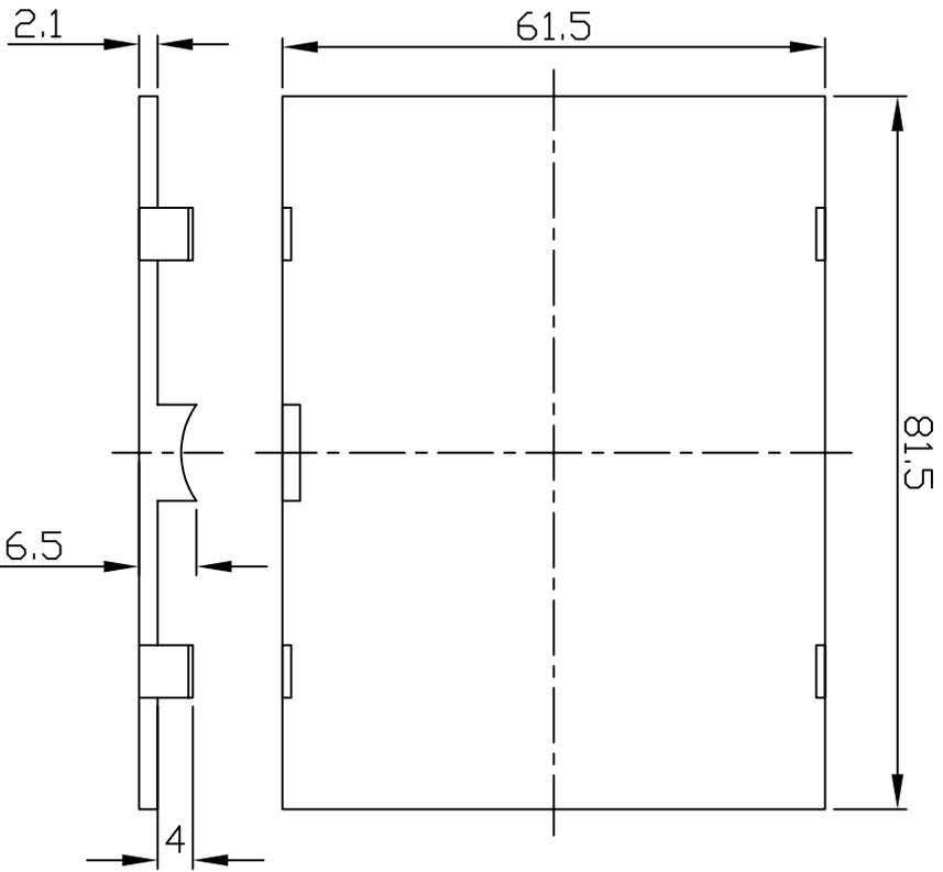
\*BLACK PLASTIC BOX WITH WALL MOUNTING BRACKET AND ONE HOLE FOR CABLE OUTLET. DIMENSION IN (mm)
