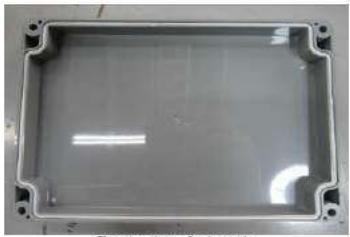
There is no trace of water inside.
