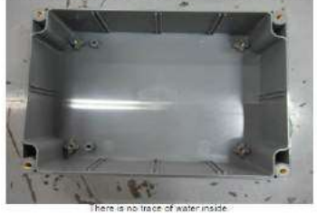
There is no trace of water inside.
